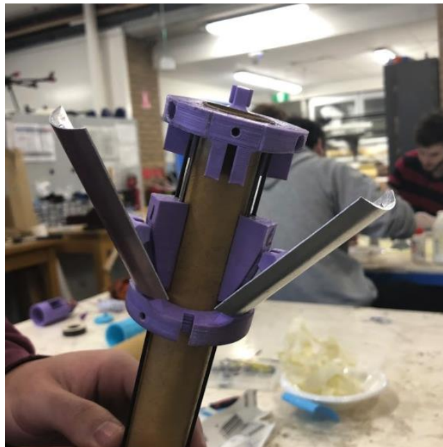
Figure 3.2.3.2: Flap actuation mechanism
