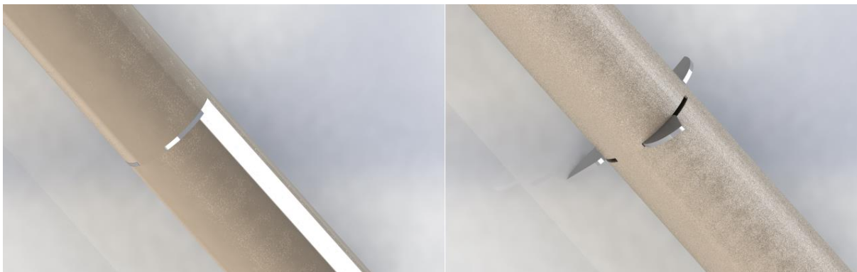
Figure 2.2: Radially deployed flaps design
