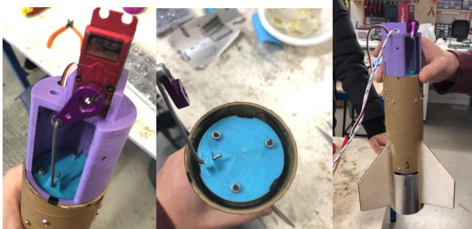
Figure 3.2.3.1: Servo connected to actuator piston (left) Actuator piston with servo linkage (middle) Assembled and powdered air brake mechanism (right)
