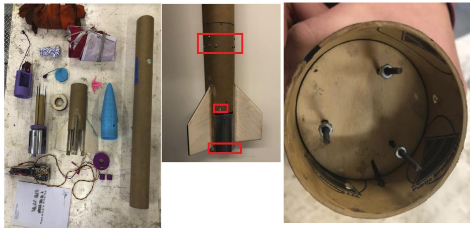
Figure 3.2.1.2: Disassembled rocket (left) fastening points (middle) motor thrust plate (right)
