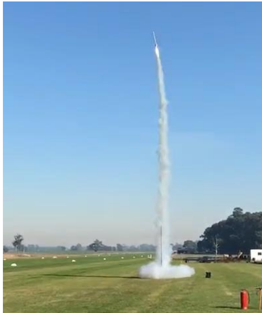
Figure 4.2.1: Rocket's initial trajectory off the rail, seen with minor slipping.
