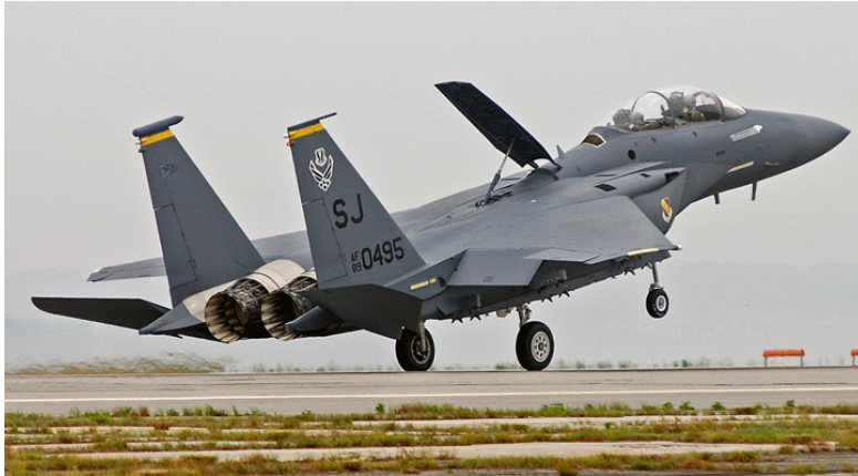
Figure 1.1.1- A McDonnell Douglas F-15 Eagle combat jet with an airbrake deployed during landing [2].
