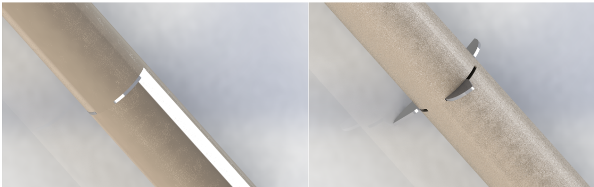
Figure 4.2.1.1: Radially actuated fins deployed (right) versus retracted (left).
